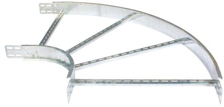
**Technical:****Product Type** Flat Bend**Width** 750mm**Height** 100mm**Weight** 9.00 Kgs**Angle** 90°**Diameter** 300mm Radius**Gauge** 1.5mm**Material** Post Hot-Dipped Galvanised (HDG)**Colour/Finish** Self Colour**Standards** BS EN ISO 1461:2009**Important:**
