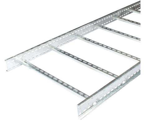
**Technical:****Product Type** Ladder Tray**Width** 750mm**Height** 100mm**Length** 3000mm**Weight** 20.30 Kgs**Dimensions** 300mm Rung Pitch**Gauge** 1.5mm**Material** Post Hot-Dipped Galvanised (HDG)**Colour/Finish** Self Colour**Standards** BS EN ISO 1461:2009**Extra Information**
