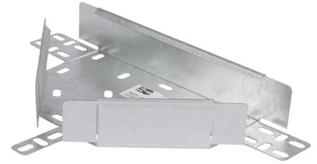
**Technical:****Product Type** Flat Tee**Width** 75mm**Height** 50mm**Weight** 0.48 Kgs**Gauge** Heavy Duty**Material** Zinc Magnesium Steel ZM310**Colour/Finish** Self Colour**Standards** BS EN 61537:2007; BS EN 10346:2015
