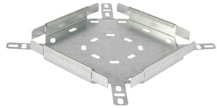
**Technical:****Product Type** Flat Fourway**Width** 75mm**Height** 25mm**Weight** 0.43 Kgs**Gauge** Medium Duty**Material** Pre-Galvanised Steel (Zinc Coated)**Colour/Finish** Self Colour**Standards** BS EN 61537:2007; BS EN 10346:2015
