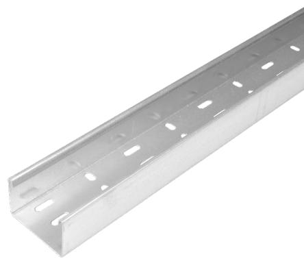
**Technical:****Product Type** Cable Tray**Width** 75mm**Height** 50mm**Length** 3000mm**Weight** 4.14 Kgs**Gauge** Heavy Duty**Material** Pre-Galvanised Steel (Zinc Coated)**Colour/Finish** Self Colour**Standards** BS EN 61537:2007; BS EN 10346:2015
