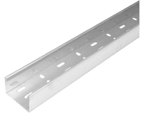
**Technical:****Product Type** Cable Tray**Width** 75mm**Height** 50mm**Length** 3000mm**Weight** 4.14 Kgs**Gauge** Heavy Duty**Material** Zinc Magnesium Steel ZM310**Colour/Finish** Self Colour**Standards** BS EN 61537:2007; BS EN 10346:2015
