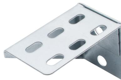
**Technical:****Product Type** Cantilever Arm**Width** 50mm**Height** 70mm**Length** 75mm**Weight** 0.20 Kgs**Gauge** Light Duty**Material** Pre-Galvanised Steel (Zinc Coated)**Colour/Finish** Self Colour**Standards** BS EN 10346:2015
