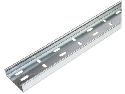
**Technical:****Product Type** Cable Tray**Width** 75mm**Height** 25mm**Length** 3000mm**Weight** 2.67 Kgs**Gauge** Medium Duty**Material** Pre-Galvanised Steel (Zinc Coated)**Colour/Finish** Self Colour**Standards** BS EN 61537:2007; BS EN 10346:2015
