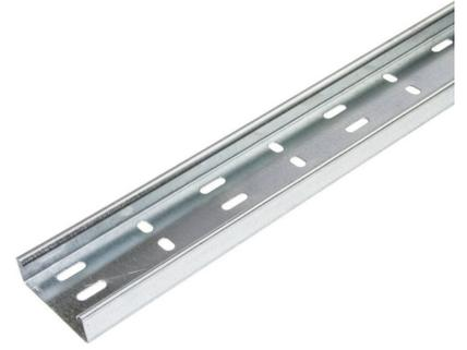
**Technical:****Product Type** Cable Tray**Width** 75mm**Height** 25mm**Length** 3000mm**Weight** 2.67 Kgs**Gauge** Medium Duty**Material** Zinc Magnesium Steel ZM310**Colour/Finish** Self Colour**Standards** BS EN 61537:2007; BS EN 10346:2015
