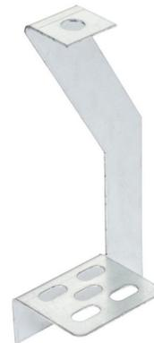
**Technical:****Product Type** Overhead Hanger**Width** 75mm**Height** 150mm**Weight** 0.13 Kgs**Material** Pre-Galvanised Steel (Zinc Coated)**Colour/Finish** Self Colour**Standards** BS EN 10346:2015
