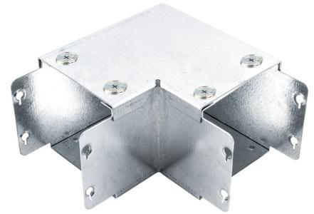
**Technical:****Product Type** Sharp Bend**Width** 75mm**Height** 75mm**Weight** 0.44 Kgs**Angle** 90°**Number of Compartments****Material** Pre-Galvanised Steel (Zinc Coated)**Colour/Finish** Self Colour**Standards** BS EN 50085-2-1 2006; BS EN 10346:2015**Important:**
