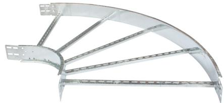
**Technical:****Product Type** Flat Bend**Width** 900mm**Height** 125mm**Weight** 12.30 Kgs**Angle** 90°**Diameter** 300mm Radius**Gauge** 1.5mm**Material** Post Hot-Dipped Galvanised (HDG)**Colour/Finish** Self Colour**Standards** BS EN ISO 1461:2009**Important:**
