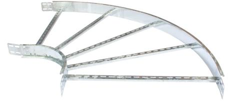
**Technical:****Product Type** Flat Bend**Width** 900mm**Height** 100mm**Weight** 11.30 Kgs**Angle** 90°**Diameter** 300mm Radius**Gauge** 1.5mm**Material** Post Hot-Dipped Galvanised (HDG)**Colour/Finish** Self Colour**Standards** BS EN ISO 1461:2009
