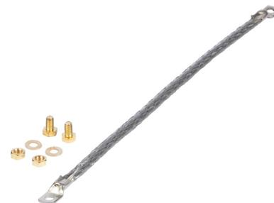
**Technical:****Product Type** Accessories**Width** 18mm**Length** 320mm**Weight** 0.01 Kgs**Gauge** 2.0mm**Material** Tinned Copper**Colour/Finish** Self Colour**Standards** BS EN ISO 1461:2009**Supplied With** 2x M6 Brass Fastener Sets Per Connector**Pack Quantity** 10 Per Pack**Important:**
