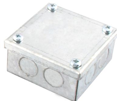
**Technical:****Product Type** Adaptable Box**Width** 75mm**Depth** 37mm**Height** 75mm**Weight** 0.22 Kgs**Material** Pre-Galvanised Steel (Zinc Coated)**Colour/Finish** Self Colour**Standards** BS EN 10346:2015**Supplied With** 20mm Knockouts
