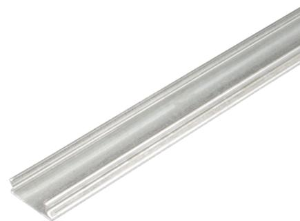
**Technical:****Product Type** Lighting Trunking Lid**Width** 50mm**Length** 2000mm**Weight** 0.66 Kgs**Material** Pre-Galvanised Steel (Zinc Coated)**Colour/Finish** Self Colour**Standards** BS EN 10346:2015
