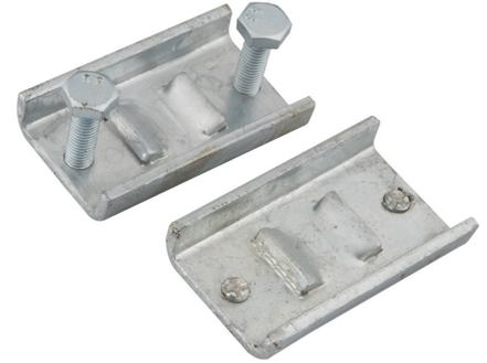
**Technical:****Product Type** Beam Clamp**Width** 89mm**Height** 55mm**Weight** 0.55 Kgs**Gauge** 6mm**Material** Post Hot-Dipped Galvanised (HDG)**Colour/Finish** Self Colour**Standards** BS 6946:1988**Supplied With** Cone pointed screw (TF050) supplied.
