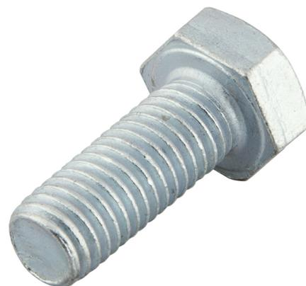
**Technical:****Product Type** Hex Set Screw**Depth** 25mm**Length** 30mm**Weight** 3.55 Kgs**Diameter** 12mm**Material** Bright Zinc Plate (BZP)**Colour/Finish** Self Colour**Standards** DIN 933**Pack Quantity** 100 Per Pack
