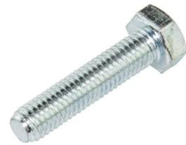
**Technical:****Product Type** Hex Set Screw**Depth** 25mm**Length** 35mm**Weight** 1.67 Kgs**Diameter** 8mm**Material** Bright Zinc Plate (BZP)**Colour/Finish** Self Colour**Standards** DIN 933**Pack Quantity** 100 Per Pack
