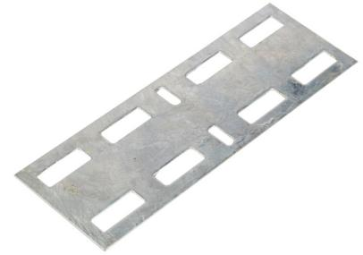
**Technical:****Product Type** Connector**Height** 84mm**Length** 250mm**Weight** 0.50 Kgs**Gauge** 1.5mm**Material** Post Hot-Dipped Galvanised (HDG)**Colour/Finish** Self Colour**Standards** BS EN ISO 1461:2009**Supplied With** 4x M10 Fastener Sets Per Coupler**Pack Quantity** Pairs**Extra Information**
