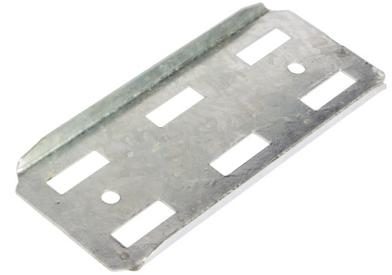
**Technical:****Product Type** Coupler**Width** 13mm**Height** 95mm**Length** 220mm**Weight** 0.60 Kgs**Gauge** 1.5mm**Material** Post Hot-Dipped Galvanised (HDG)**Colour/Finish** Self Colour**Standards** BS EN ISO 1461:2009**Supplied With** 4x M10 Fastener Sets Per Coupler**Pack Quantity** Pairs**Extra Information**
