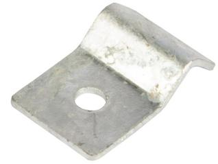
**Technical:****Product Type** Hold Down Clip**Width** 40mm**Height** 15mm**Length** 65mm**Weight** 0.07 Kgs**Dimensions** One Hole 11mm**Gauge** 1.5mm**Material** Post Hot-Dipped Galvanised (HDG)**Colour/Finish** Self Colour**Standards** BS EN ISO 1461:2009**Pack Quantity** Single
