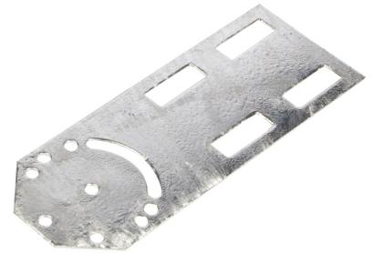
**Technical:****Product Type** Connector**Height** 80mm**Length** 212mm**Weight** 0.80 Kgs**Angle** 15° | 18° | 22.5° | 30° | 45°**Gauge** 1.5mm**Material** Post Hot-Dipped Galvanised (HDG)**Colour/Finish** Self Colour**Standards** BS EN ISO 1461:2009**Supplied With** 2x M10 Fastener Sets Per Connector 3x M6 setscrews**Pack Quantity** Pairs (4x Plates)**Important:**
