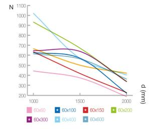
$AWL = (Newtons/m) \; ; \; d = distance \; between \; supports \; (mm) \\ 1 \; Newton = 0.102 \; kg. \\$
