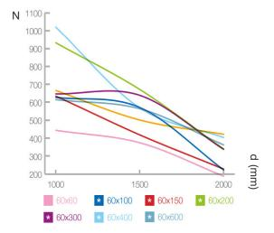
AWL = (Newtons/m); d = distance between supports (mm) 1 Newton = 0.102 kg.
