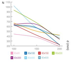
$<sup>\</sup>label{eq:AWL} \begin{array}{l} AWL = (Newtons/m) \ ; \ d = distance \ between \ supports \ (mm) \\ 1 \ Newton = 0.102 \ kg. \end{array}$
