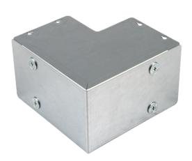
Cable trunking is designed such that the main body carries the weight of cables. Trunking should NOT be installed in any way that causes the lid to carry the cable
